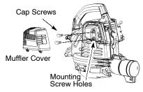
**NOTE:** The muffler mounting screws are located behind the cap screws. The cap screws must be removed to access the mounting screws.
